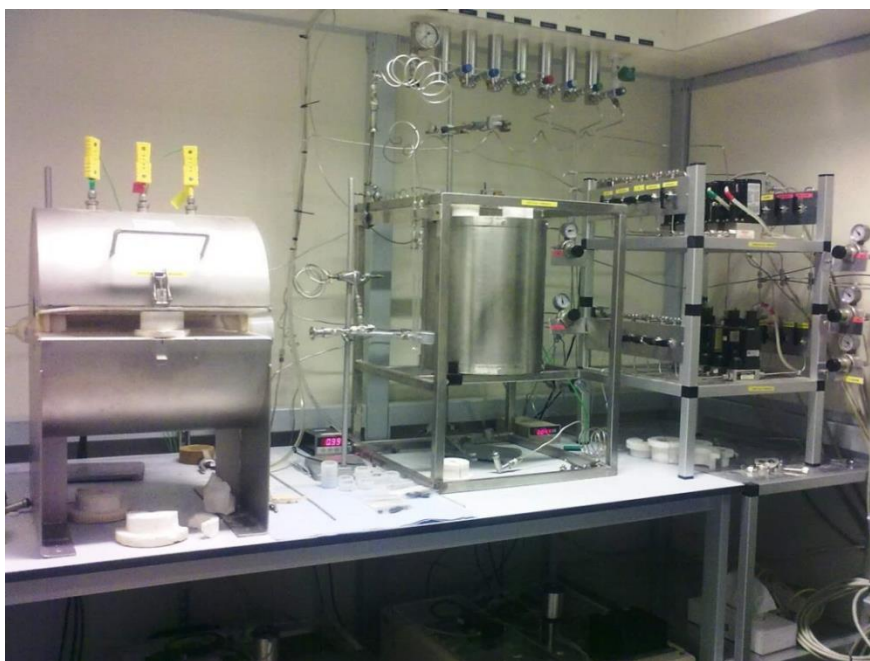
Figure 3: A photograph of the CVD setup for carbon nanofiber growth.
