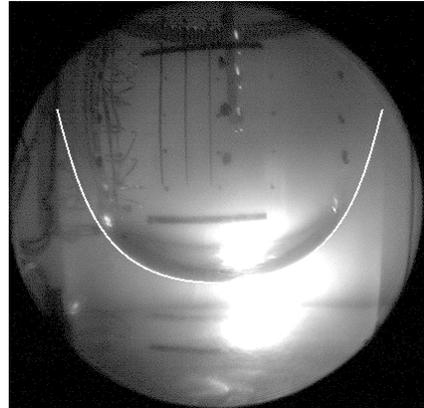
Figure 2: Intermediate surface contour of liquid hydrogen in a gaseous hydrogen environment. The free surface is highlighted in white. The static contact angle is zero but the tangent at the wall is not visible due to optical distortions of the cylindrical container wall.
