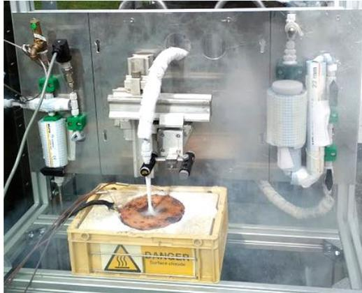
Experimental set-up, Projection of cryogenic fluids onto a heated copper target
