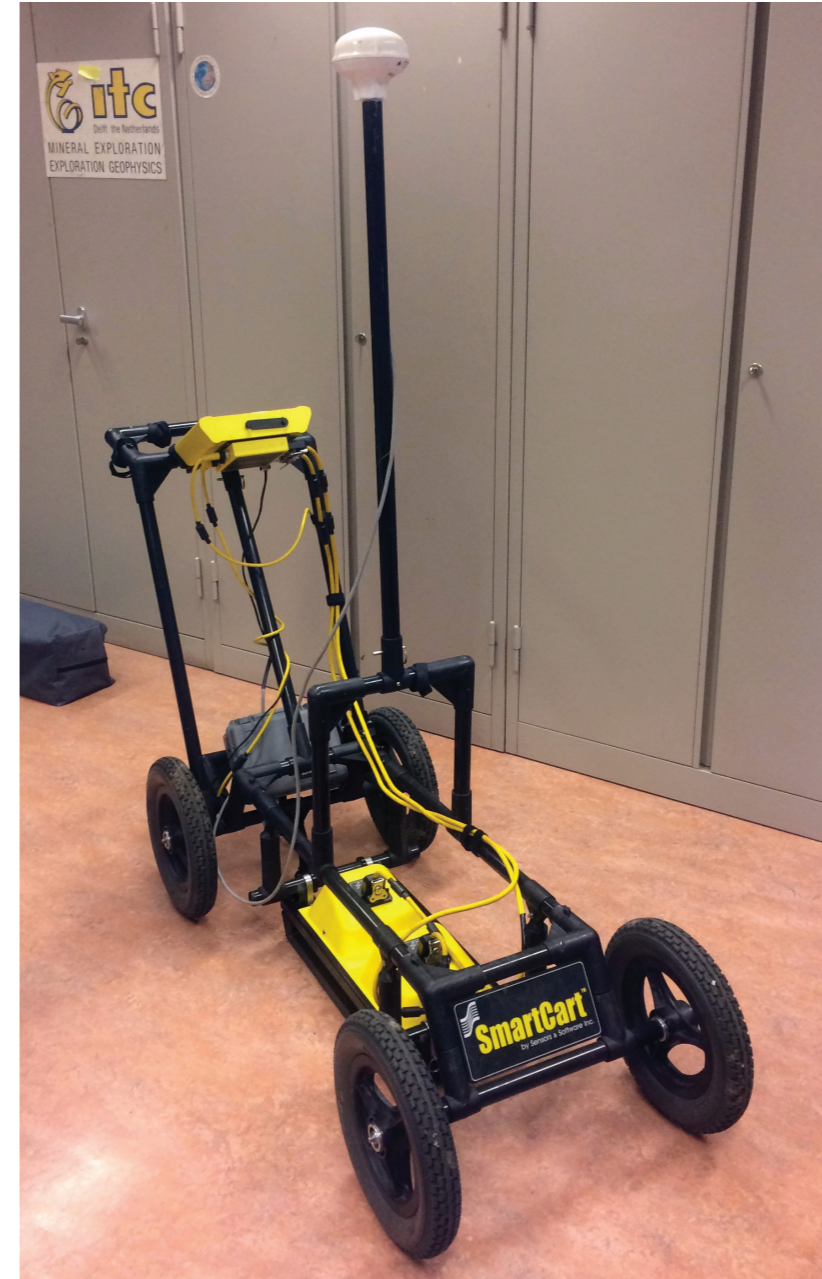
Figure 1. Sensors and software GPR Pulse EKKO Pro mounted with 500MHz transducers, and possibility to mount 100MHz antennas. GPR lines are collected perpendicular and parallel to the direction of the rad.
