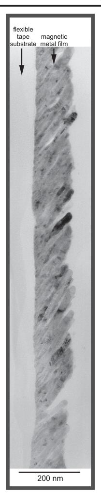
XTEM specimen preparation can be challenging for, e.g., samples composed of materials with very different properties, such as the example given in this application note. It displays a TEM image at low magnification of a brittle metal film with columnar structure (CoCr) which was deposited on a flexible plastic tape (PET).
