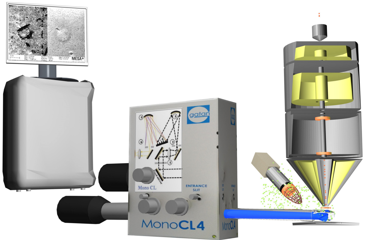
Figure 3. Illustration showing the complete path of the electrons in the SEM to the imaging of the CL and SE signals on the SEM monitor
