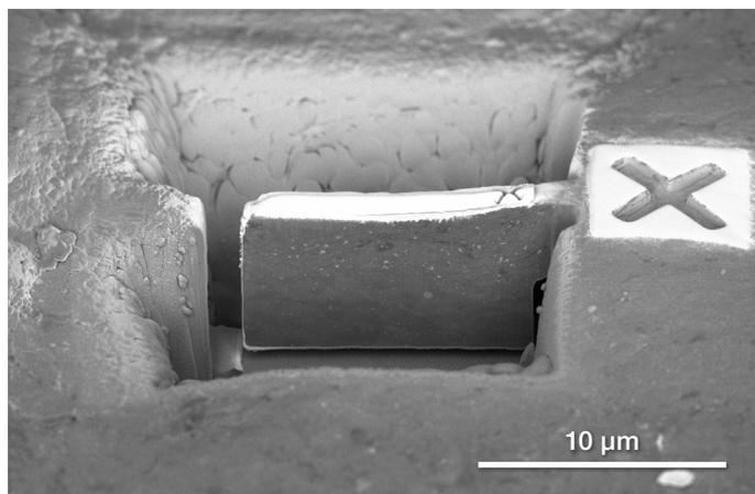
Figure 2.2. Example of a sample after chunking and undercut, ready for *in situ* lift-out. The large fiducial on the side is used for chunking automation, while the smaller one on the lamella will be used later for final thinning automation.
