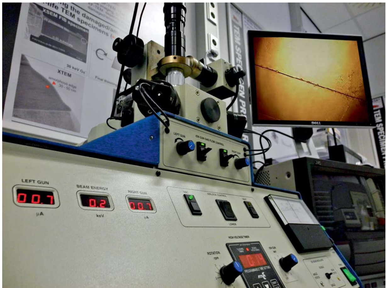
Fig. 3: GATAN model 691 dual-beam ion miller in action at MESA+ NanoLab. The Argon ion beam energy can be adjusted in the energy range of 6 - 0.1 keV. The PIPS, as the instrument is commonly named, is used to obtain final electron transparency of TEM specimens pre-thinned by mechanical polishing techniques, such as Dimple Grinding /
