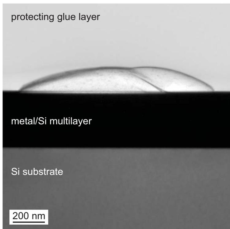
*Fig. 1: TEM cross-section revealing a fully intact double-blister with diameter of the order of  $1.5\ \mu\text{m}$ . The specimen thickness at this stage is estimated to be at least  $1.5\ \mu\text{m}$ , allowing to observe the fully intact hemispherical half-dome of the double-blister though. Individual layers are however, barely visible.*
