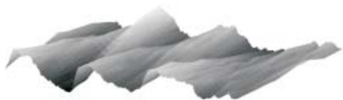
Fig. 1. Alternate bars in a channel as measured in a straight laboratory flume Lanzoni [9]. The crests alternate between the side banks. (The flow is from right to left.)
