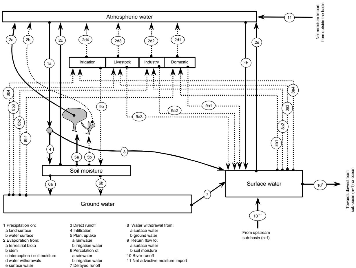
Fig. 4. Water flow schematisation within a sub-basin.
