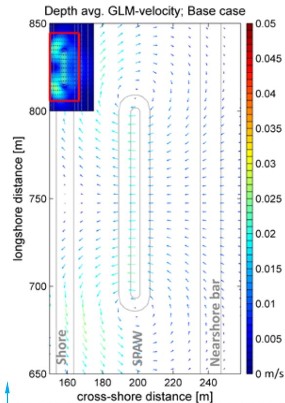
FIG. 4 Top view of depth-averaged Generalized Lagrangian Mean velocity pattern around the SPAW location. Vectors show directions and magnitude, contour lines show bottom contours.
