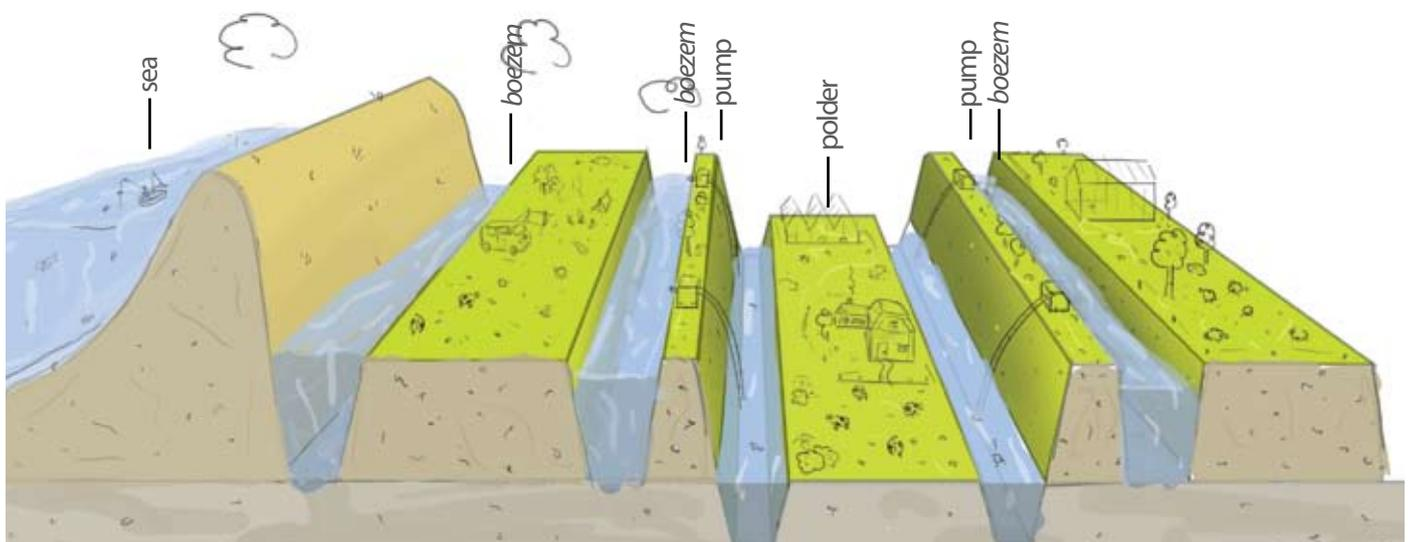
Figure 1: Water systems in the lower parts of the Netherlands consist of polders below sea level, from which water is pumped to the boezemwater. Boezem pumping stations drain into the rivers or the sea.
