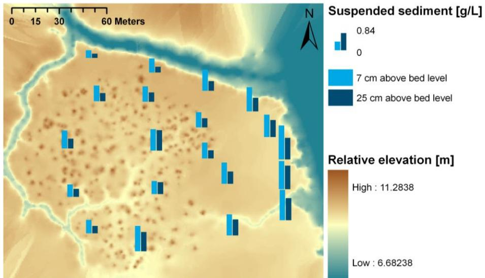
Figure 7 Suspended sediment concentrations (in g/L) at all elevated grid points measured at 7 cm (light blue) and 25 cm (dark blue) above bed level. Suspended sediment concentrations are averaged over 2 spring tides.
