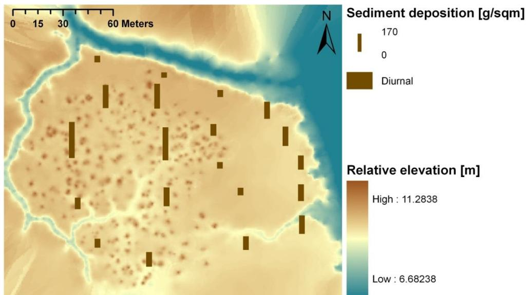
Figure 8 Sediment deposition rates (in g/m<sup>2</sup>) at all elevated grid points measured. Sediment deposition rates are averaged over 2 spring tides.
