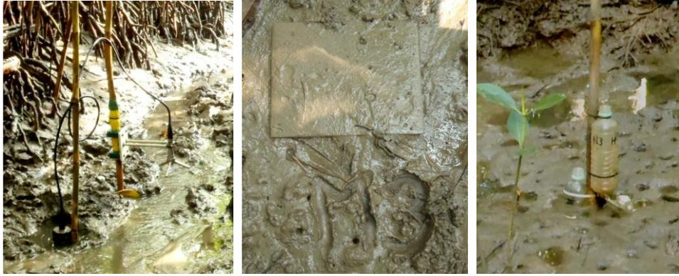
Figure 3 From left to right: Deployment of an ADV at P1; a sediment trap after 1 day out in the field at M3 and SSC samples taken at N3
