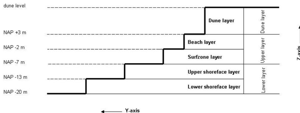
Figure 5. 'Block' representation of coastal profile in PONTOS (Steezel & Wang, 2003)
