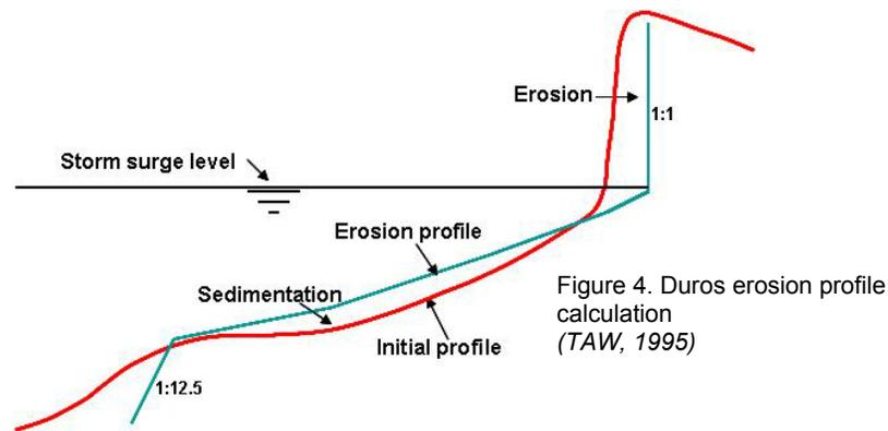
Figure 4. Duros erosion profile calculation (TAW, 1995)
