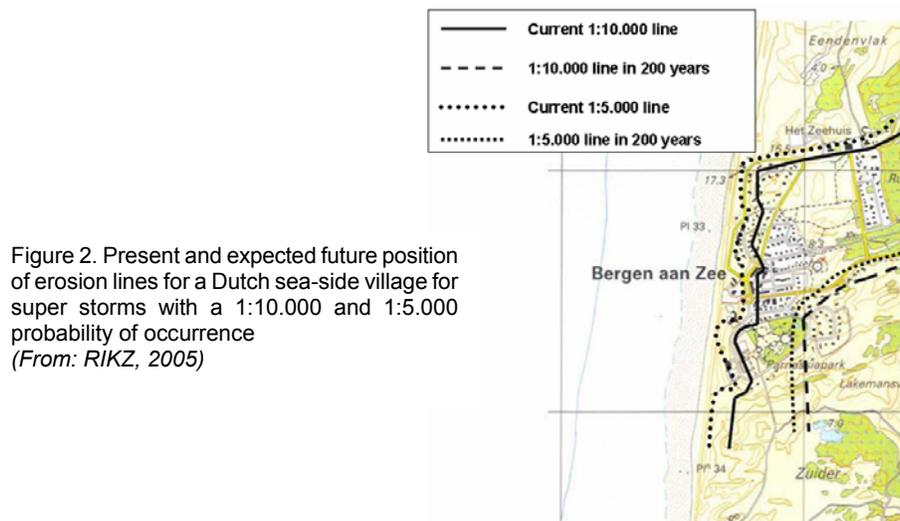
Figure 2. Present and expected future position of erosion lines for a Dutch sea-side village for super storms with a 1:10.000 and 1:5.000 probability of occurrence (From: RIKZ, 2005)
