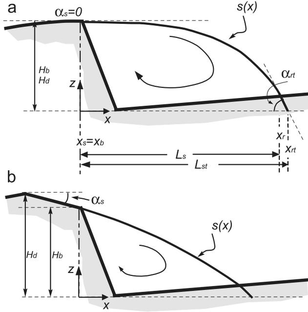
**Figure 1.** Schematic representation of flow separation in the lee of a dune with (a) horizontal bed at the flow separation point and (b) negative bed slope at the flow separation point, including a sketch of the separation streamline. Flow separation is assumed to occur at the brink point ( $x_b$ ). See the notation section for used parameters.
