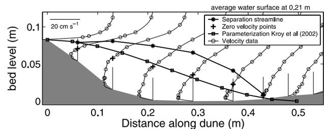
**Figure 2.** Illustration of velocity data, zero velocity points, and separation streamline for experiment T5 of Van Mierlo and De Ruiter [1988]. The separation streamline is compared to the parameterization of Kroy et al. [2002].
