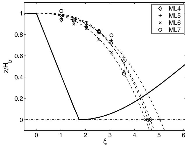
**Figure 3.** Separation streamlines for data of *McLean et al.* [1999]. Dashed lines are the regressed separation streamlines (symbols at trough elevation distinguish the four experiments).
