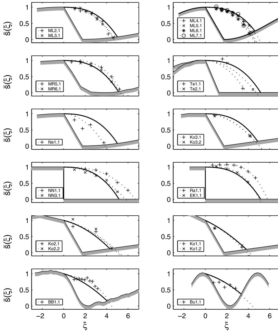
**Figure 6.** Comparison of the parameterization with the separation streamlines found from the regression analysis. Bed profiles are underlain by a gray shading for clarity. Within the flow separation zone the solid lines represent the parameterization, the symbols represent the measured vertical positions along the separation streamlines ( $z_{sep}$ ), and the dotted line represents the fitted separation streamlines to these positions.
