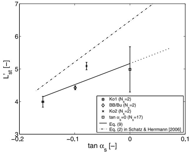
**Figure 5.** Nondimensional length of the flow separation zone ( $L'_{st}$ ) as a function of the bed slope at the flow separation point ( $\tan \alpha_s$ ). The data are grouped into four slope classes with  $N_s$ , the number of observations in that class; per class the mean and its standard deviation are shown. The solid line is a linear fit through the mean nondimensional separation zone lengths, and the dash-dotted line is equation (2) of *Schatz and Herrmann* [2006].
