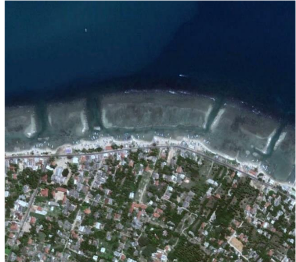
Figure 8: Sandy coastline influenced by the construction of a series of small jetties and positioned behind interrupted reefs at Point Pedro (Google Earth).
