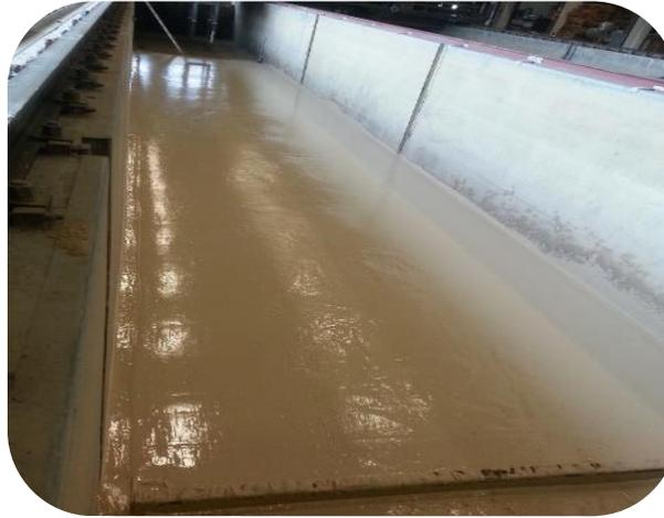
Figure 50: Prepared sediment bed.
