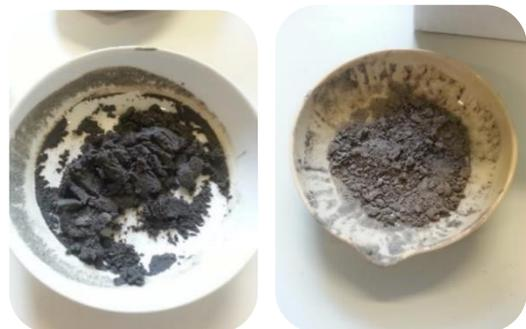
Figure 48: (Left) clayey soil sample tube 2. (Right) sandy soil sample tube 7.
