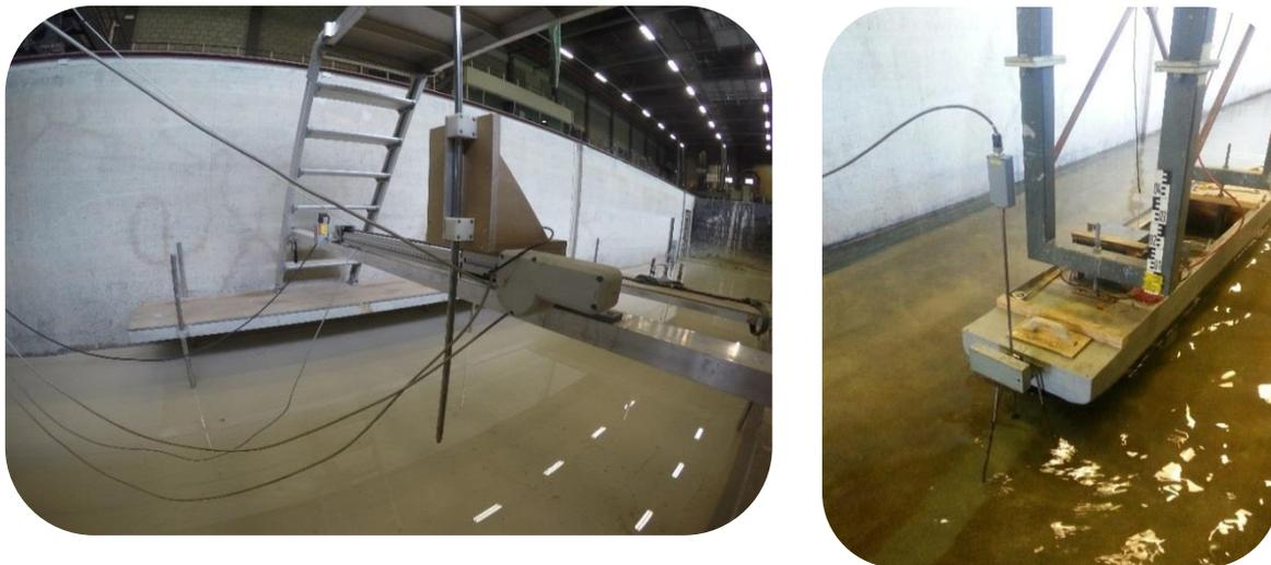
Figure 12: (Left) movable echo sounder; (Right) EMS measuring propeller wash.
