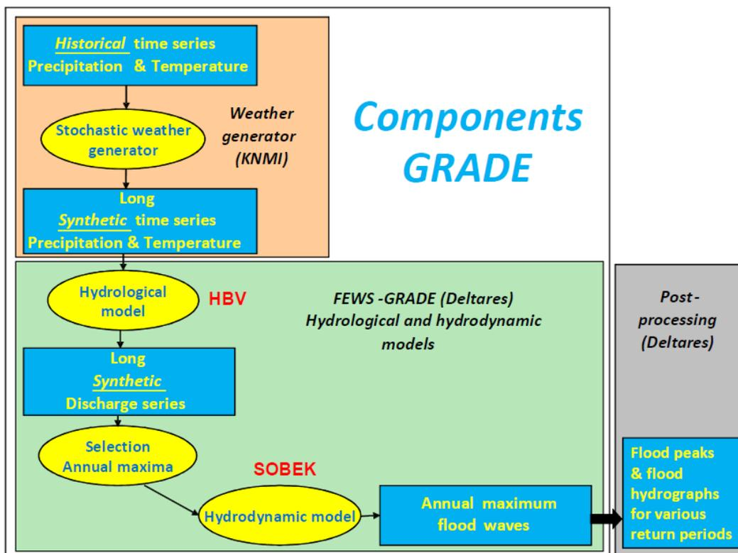
Figure 4 Components of GRADE (Hegnauer et al., 2014)
