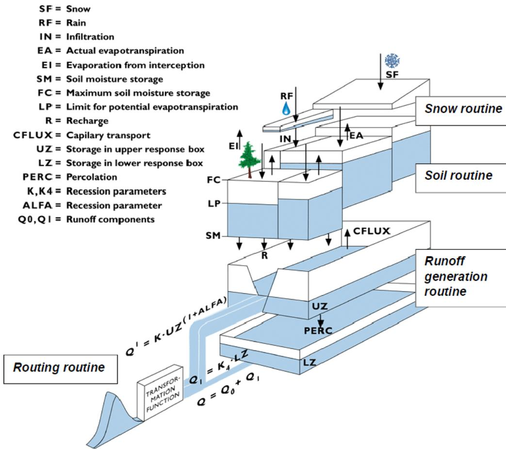
Figure 6 Schematic presentation of the HBV model for one sub-catchment (Hegnauer et al. (2014) after Lindstrom et al. (1997)).
