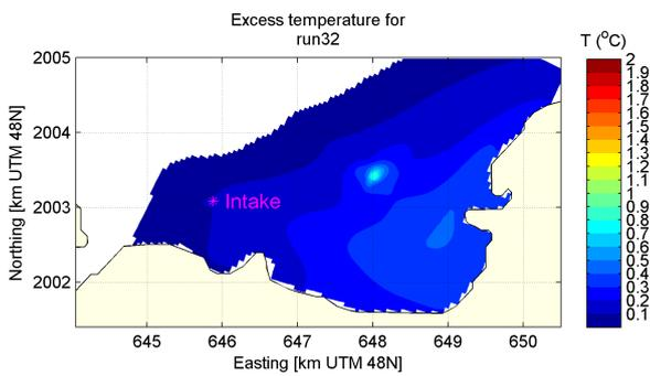
(c) Mean temperature in intake layer, 5cm/s SE current with  $Q=0m^3/s$
