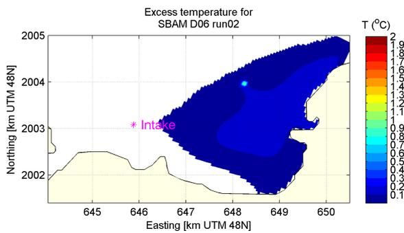
(c) Mean temperature in intake layer, 5cm/s SE residual current
