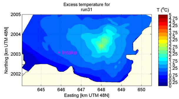
(b) Maximum temperature in surface layer, 3cm/s NW current with  $Q=0m^3/s$
