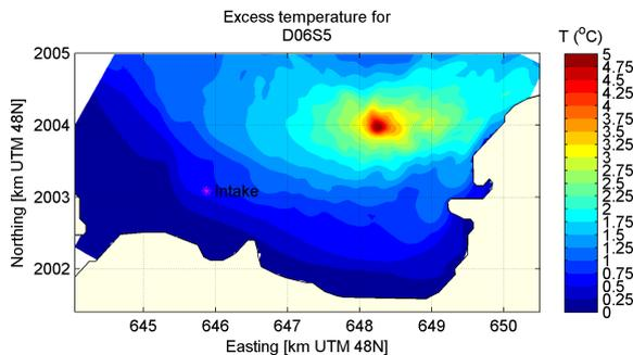
Figure 5.10: Maximum excess temperature in surface layer for design 6 and scenario 5, Approach A
