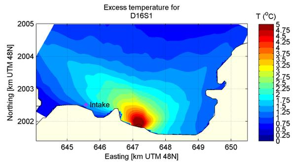
Figure 5.18: Maximum excess temperature in intake layer for design 16, Approach B
