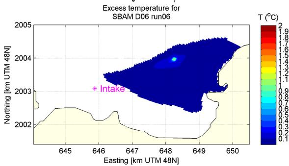
(e) Mean temperature in intake layer,  $Q=170m^3/s$
