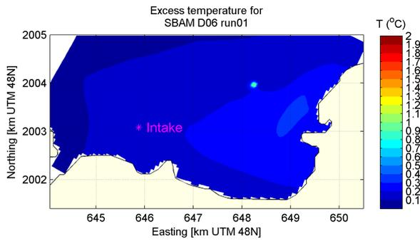
(a) Mean temperature in intake layer, 3cm/s NW residual current
