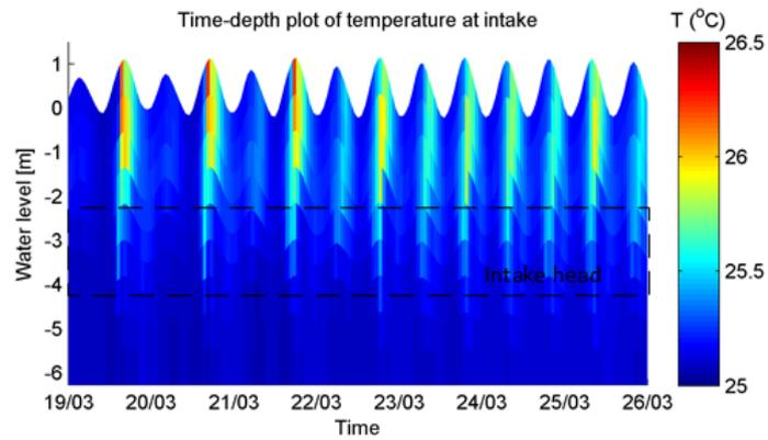
Figure 5.9: Depth-time plot at the intake for  $70m^3/s$  and a NW current, design 8.
