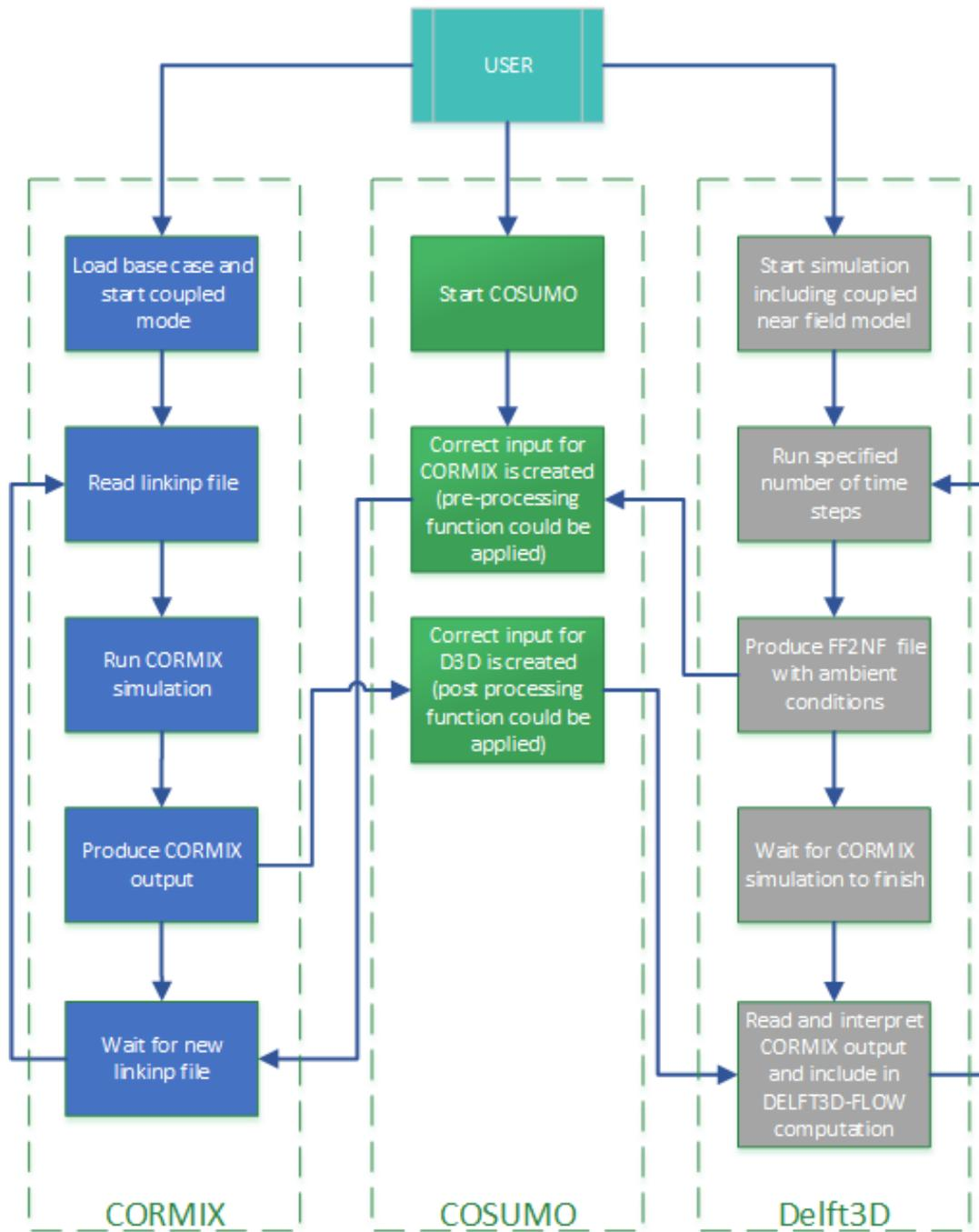
Figure 4.6: Flow chart showing the CORMIX-COSUMO-Delft3D interaction for the two-way coupling method.
