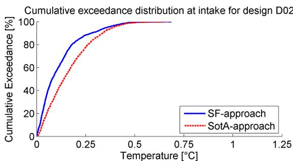
Figure 5.12: Yearly excess intake temperature for both approaches found for Design 2
