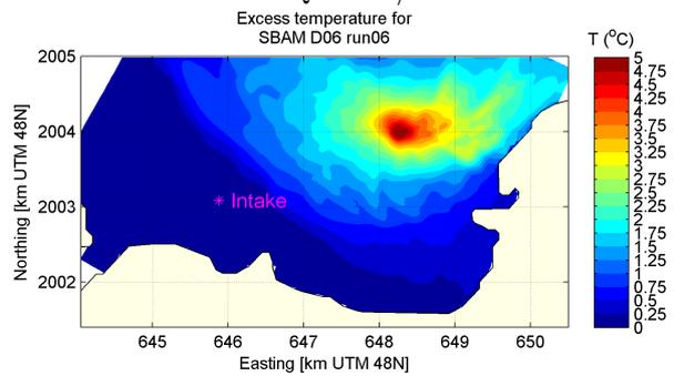
(f) Maximum temperature in surface layer,  $Q=170m^3/s$
