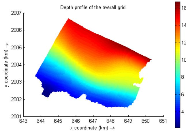
Figure 4.4: Depth profile of refined area of the grid.
