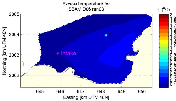
(a) Mean temperature in the intake layer, no residual current
