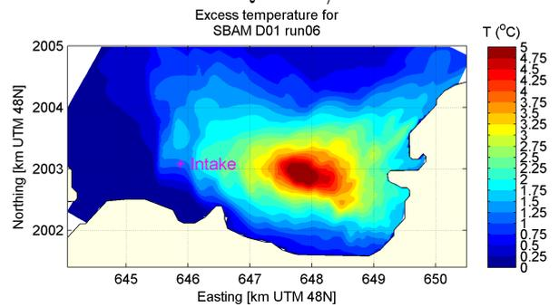
(f) Maximum temperature in surface layer,  $Q=170m^3/s$
