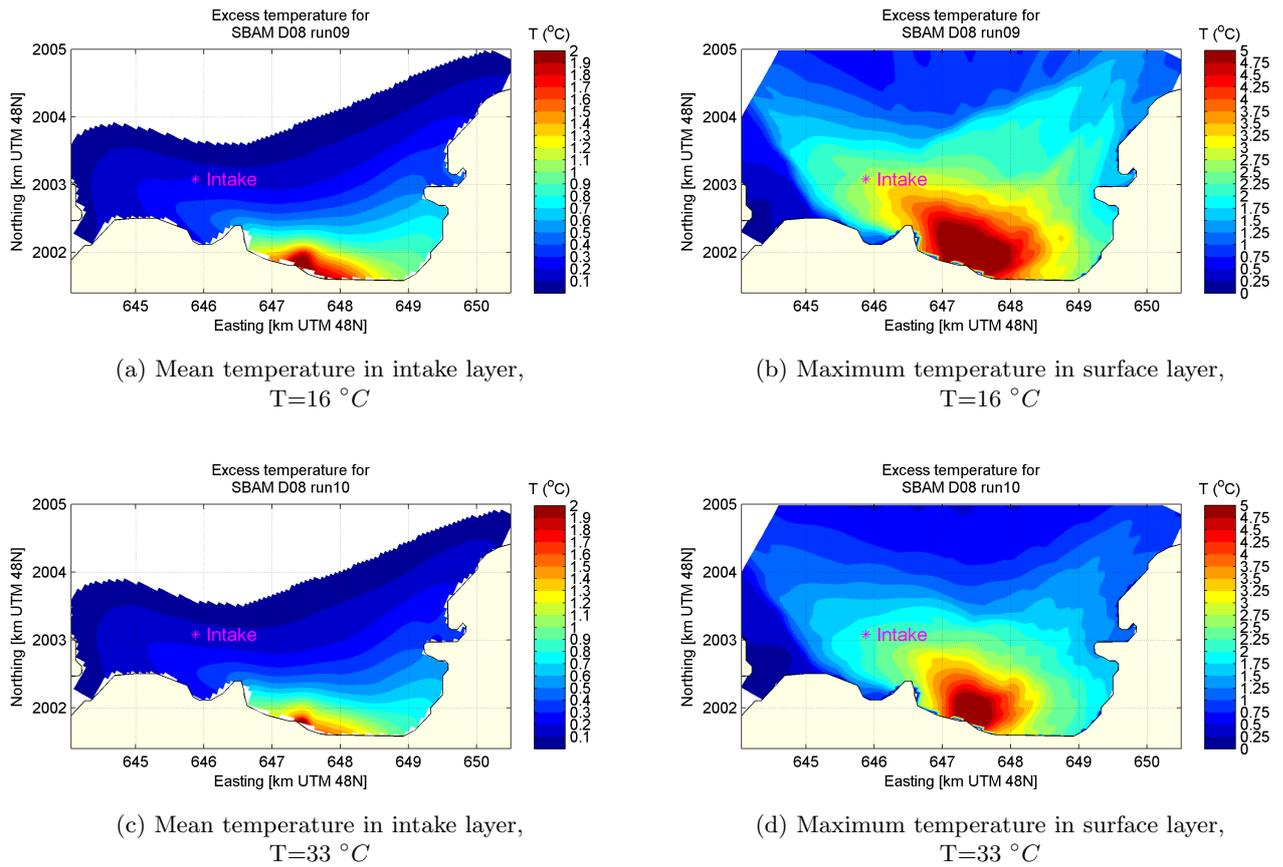
Figure A.12: Influence of the ambient temperature on system behavior for design 8. For left pictures, the excess temperatures below 0.05 are marked in white to highlight the extent of the plume. Note the scale differences.
