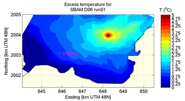
(b) Maximum temperature in surface layer, 3cm/s NW residual current
