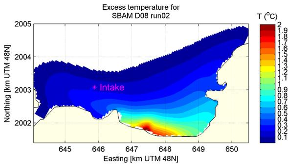
(a) Mean temperature in intake layer, persistent wind
