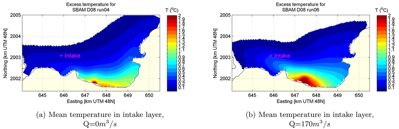
Figure 5.1: Example of the plume trapping by the river, represented by the mean temperature at the intake layer for a surface outfall. Excess temperatures below 0.05 are marked in white to highlight the extent of the plume.
