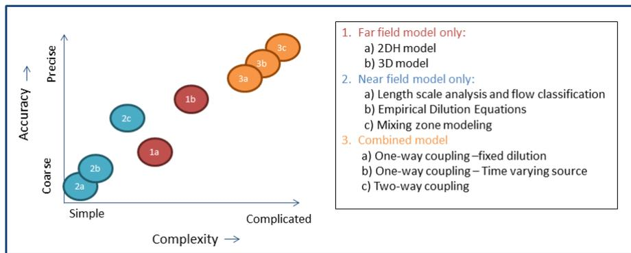
Figure 2.1: Very rough comparison of the available models to assess the plumes behavior. Please note that the accuracy is highly dependent on the ambient characteristics.
