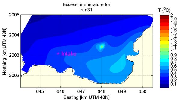
(a) Mean temperature in intake layer, 3cm/s NW current with  $Q=0m^3/s$
