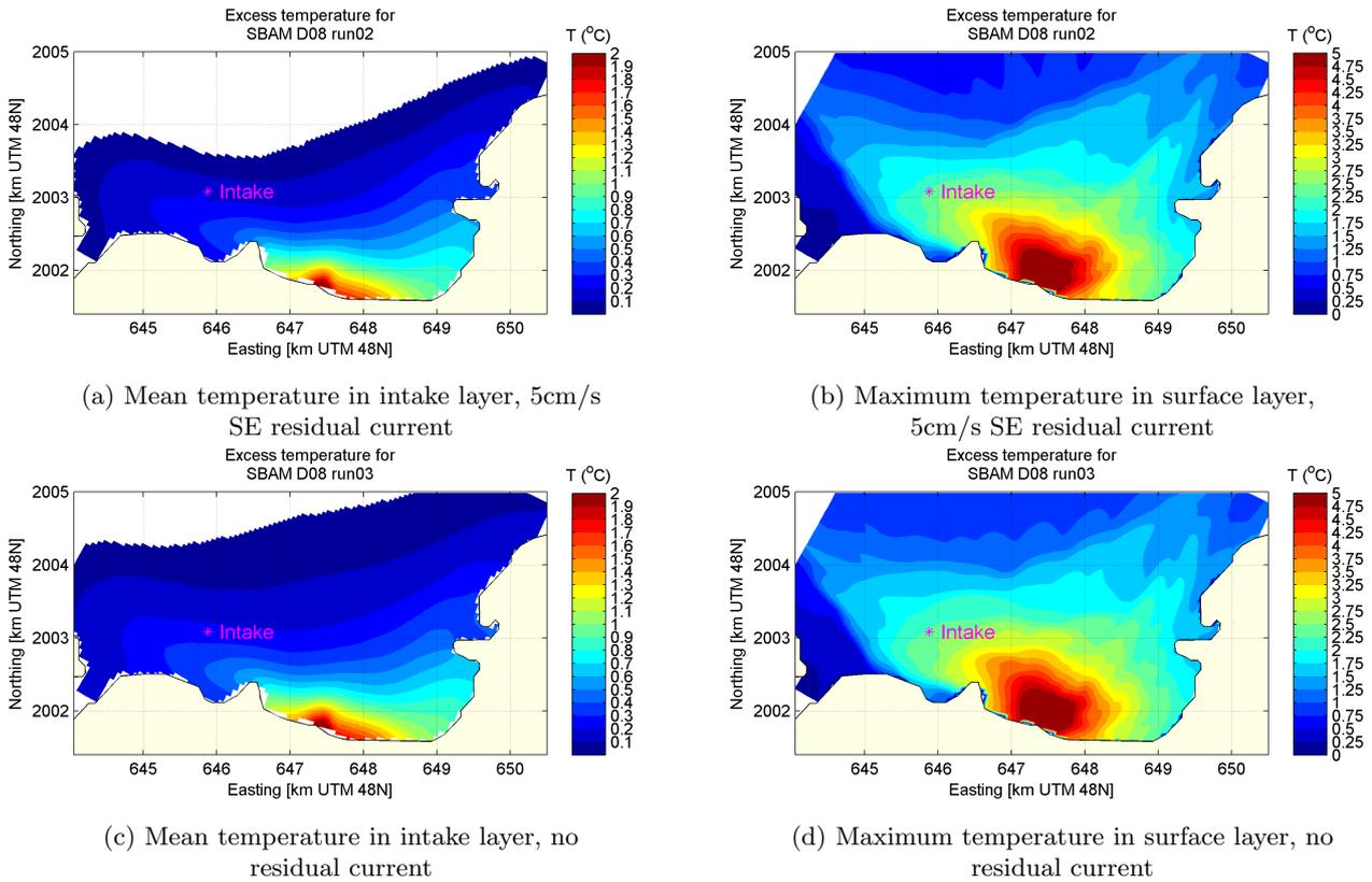
Figure A.3: Influence of the residual current on system behavior for design 8. For left pictures, the excess temperatures below 0.05 are marked in white to highlight the extent of the plume. Note the scale differences.
