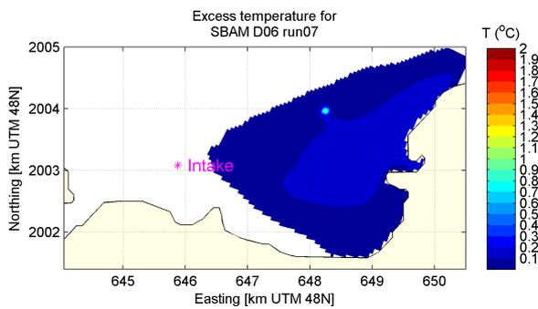
(c) Mean temperature in intake layer, maximum wind
