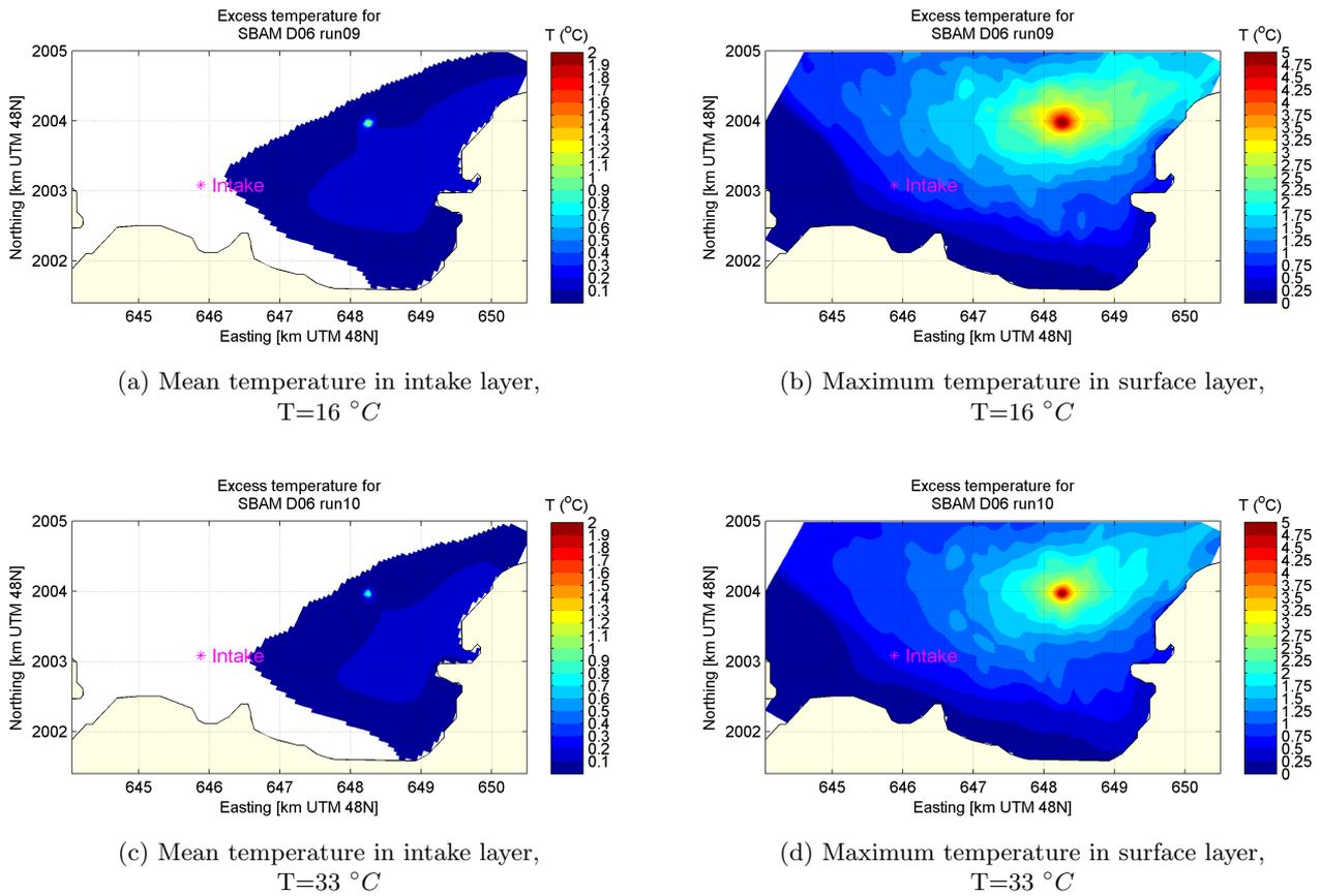
Figure A.11: Influence of the ambient temperature on system behavior for design 6. For left pictures, the excess temperatures below 0.05 are marked in white to highlight the extent of the plume. Note the scale differences.
