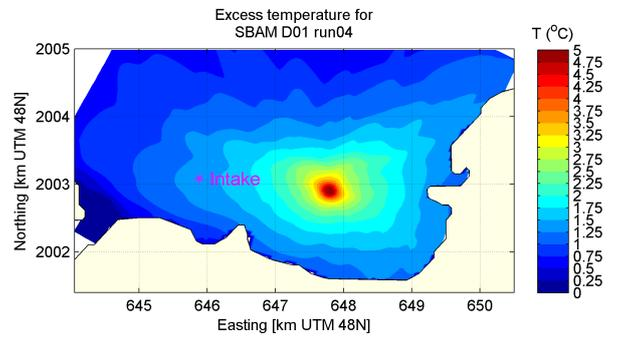
(b) Maximum temperature in surface layer,  $Q=0m^3/s$
