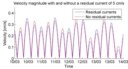
Figure 4.5: Model with and without residual current, example location in the North-West.
