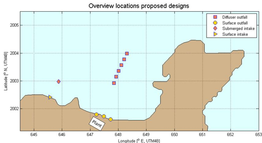
Figure 3.9: Overview of used locations of the different designs in the optimization process.
