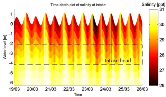
Figure 5.3: Depth-time plot at the intake for  $70m^3/s$ , middle open outfall design (8).
