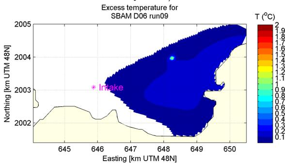
(e) Mean temperature in intake layer,  $T=16^\circ C$
