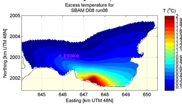
(e) Mean temperature in intake layer,
