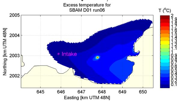
(e) Mean temperature in intake layer,  $Q=170m^3/s$
