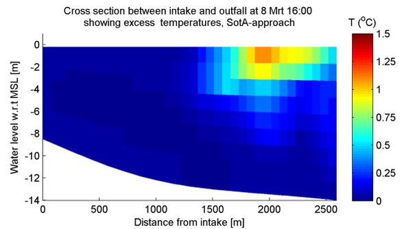
Figure 5.15: Cross section from intake to outfall, showing the the excess temperature at 8 March 16:00 for Design 5, scenario 5, Approach B.
