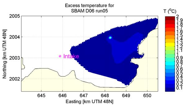
(c) Mean temperature in intake layer,  $Q=70m^3/s$
