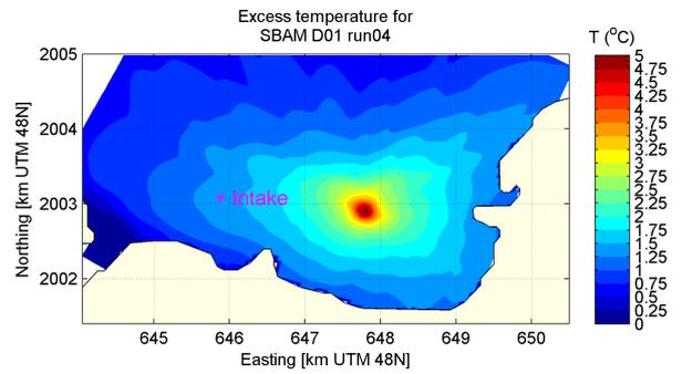
(b) Maximum temperature in surface layer,  $Q=0m^3/s$
