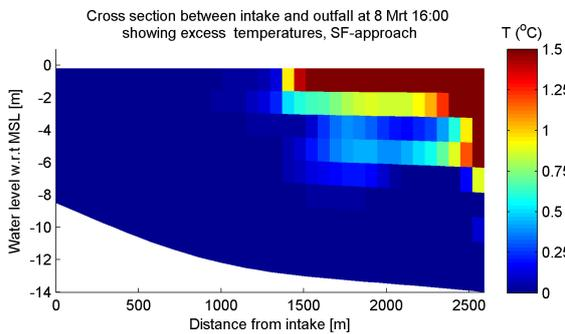
Figure 5.14: Cross section from intake to outfall, showing the the excess temperature at 8 March 16:00 for Design 5, scenario 5, Approach A.
