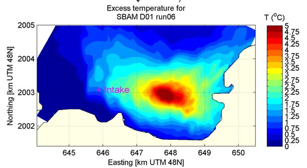
(f) Maximum temperature in surface layer,  $Q=170m^3/s$
