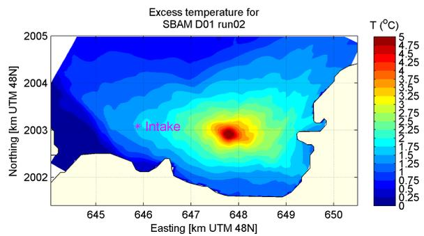
(d) Maximum temperature in surface layer, 5cm/s SE residual current
