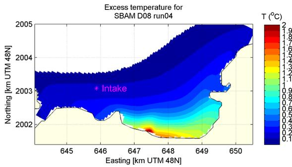
(a) Mean temperature in intake layer,
