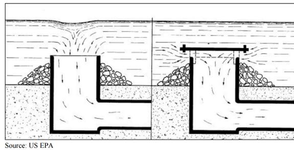
Figure 5.16: The submerged intake as modeled (left) and the reality (right)
