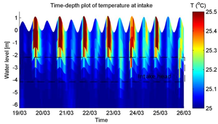
Figure 5.2: Depth-time plot at the intake for  $70m^3/s$ , middle open outfall design (8).
