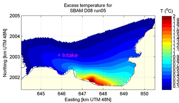
(c) Mean temperature in intake layer,
