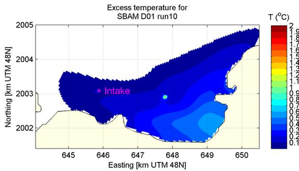
(c) Mean temperature in intake layer,
