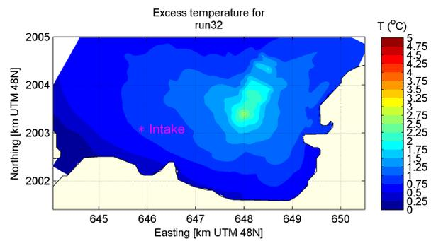
(d) Maximum temperature in surface layer, 5cm/s SE current with  $Q=0m^3/s$
