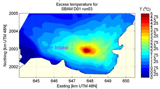
(f) Maximum temperature in surface layer, no residual current
