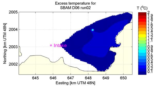
(b) Mean temperature in the surface layer, 5cm/s SE residual current
