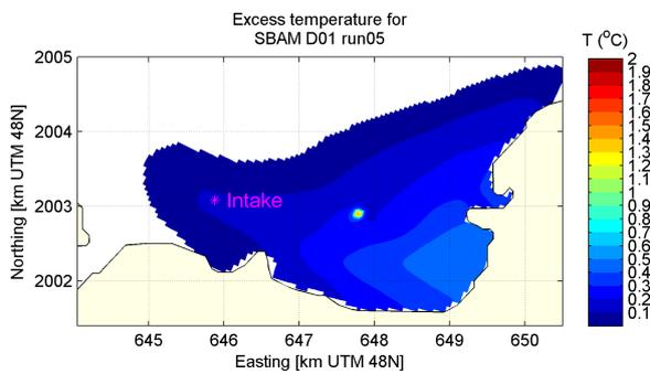
(c) Mean temperature in intake layer,  $Q=70m^3/s$
