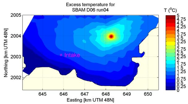
(b) Maximum temperature in surface layer,  $Q=0m^3/s$
