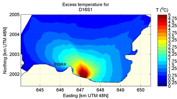
Figure 5.17: Maximum excess temperature in intake layer for design 16, Approach A
