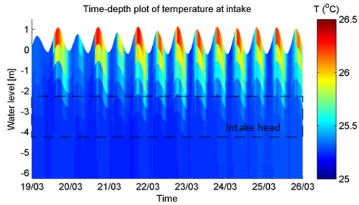
Figure 5.8: Depth-time plot at the intake for  $0m^3/s$  and a NW current, design 8.
