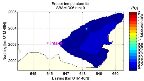
(f) Mean temperature in intake layer,  $T=33^\circ C$
