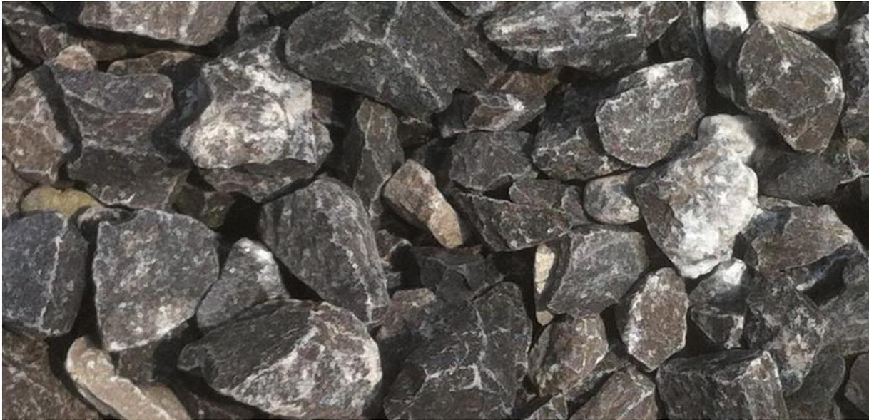
Appendix figure 1 Loose rock which can function as bed protection (Stenen, 2015)
