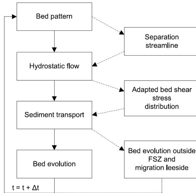
FIGURE 2: SETUP OF THE PARAMETERIZED DUNE MODEL (AFTER PAARLBERG ET AL., 2009)
