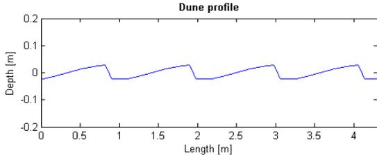
FIGURE 3: DUNE PROFILE OF FOUR IDENTICAL DUNES AS PREDICTED BY THE PARAMETERIZED DUNE MODEL, FLOW DIRECTION FROM LEFT TO RIGHT
