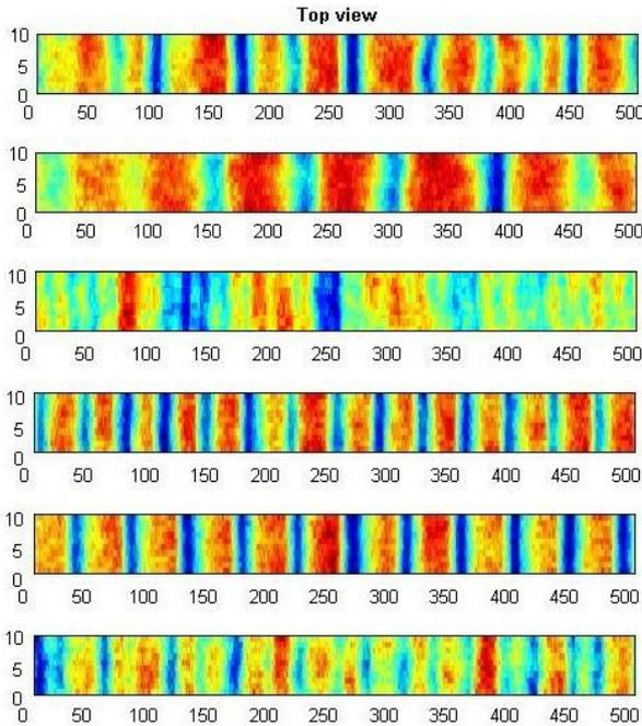
FIGURE 13: TOP VIEW BOTTOM PROFILE CHANGING STEP LENGTH, (IN ORDER: 8, 15, 20, 40, 50 AND 60) VALUES ON X AXIS IN NUMBER OF CELLS, FLOW DIRECTION FROM LEFT TO RIGHT
