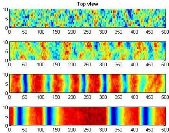
FIGURE 11: TOP VIEW BOTTOM PROFILE CHANGING SLOTS, (IN ORDER 12.5, 37.5, 100 AND 5000 ( $\cdot 10^3$ )) VALUES ON AXIS IN NUMBER OF CELLS, FLOW DIRECTION FROM LEFT TO RIGHT
