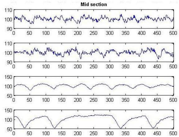
FIGURE 12: MID SECTION BOTTOM PROFILE CHANGING SLOTS, (IN ORDER 12.5, 37.5, 100 AND 5000 ( $\cdot 10^3$ )) VALUES ON AXIS IN NUMBER OF CELLS, FLOW DIRECTION FROM LEFT TO RIGHT
