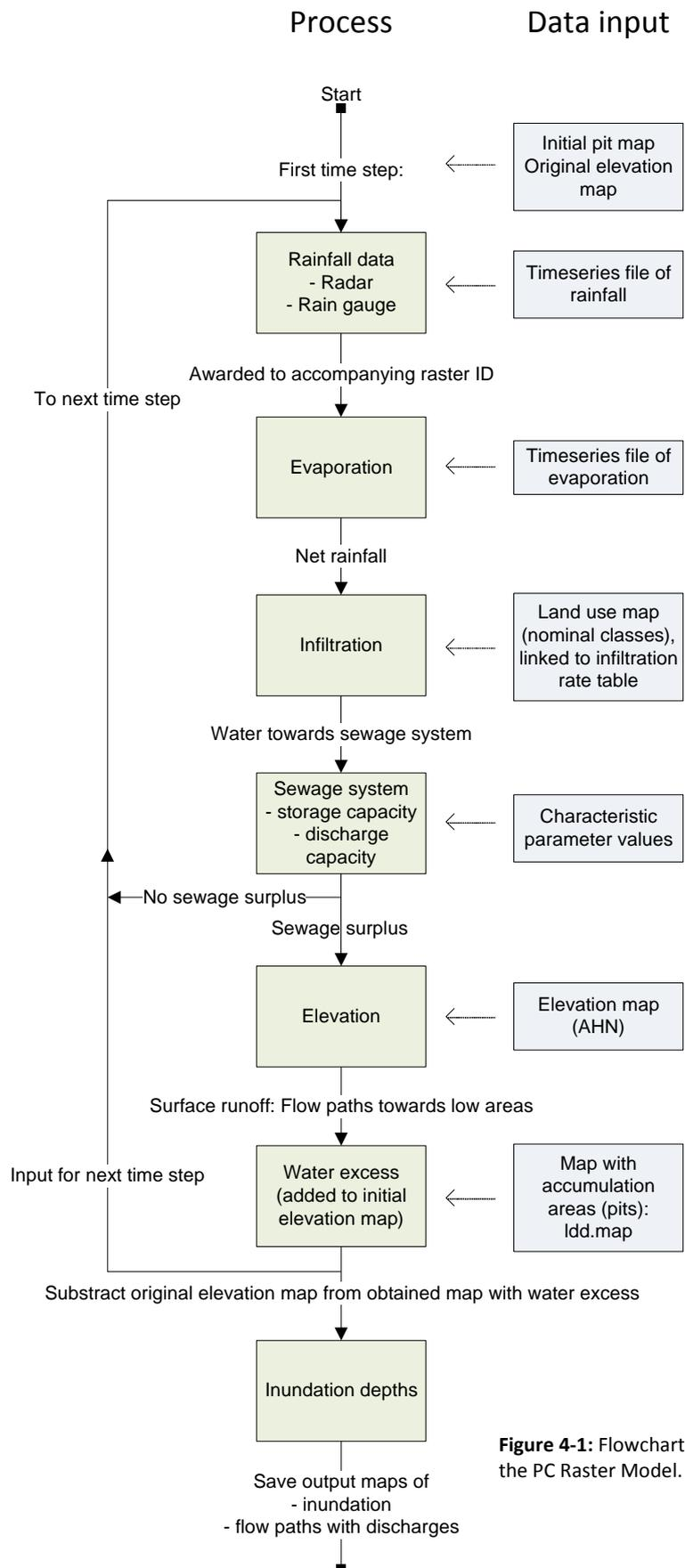
Figure 4-1: Flowchart of the PC Raster Model.
