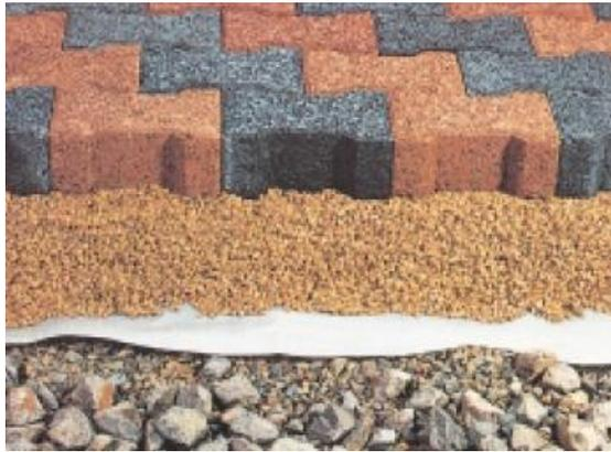
**Figure 6-1:** Porous blocks laid on a bed of ground and crushed stone. The sub surface layers provide useful storage volume for extreme rainfall events.
