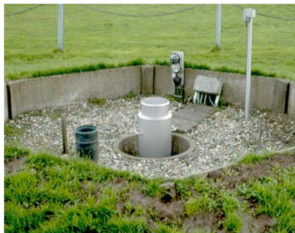
**Figure 1-1:** Left: Weather radar of the KNMI in De Bilt (picture by Iwan Holleman, KNMI). Right: Automatic rain gauge of the KNMI (KNMI, 2009).
