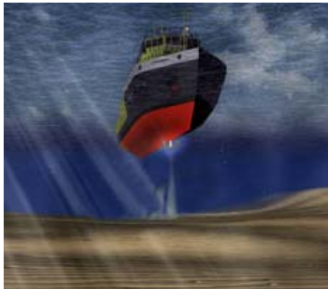
Fig. 6: Single-beam loding [RWS, 2005]
