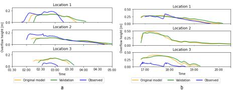
Figure 1 Temporal validation for rainfall events 1 (a) and 2 (b). Overflow height is the water level downstream of a sewage overflow location. Simulation results are close to the original model. Simulations at Location 3 do not match observed values. For Location 2 in Figure b, no observational data was available.
