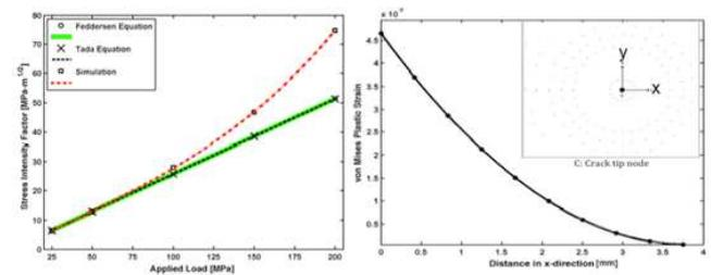
Figure 3 : Stress intensity calculation (left), von Mises plastic strain profile in x-direction (right)
