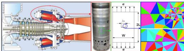
Figure 1 : Fracture-mechanics on gas turbine liner.
