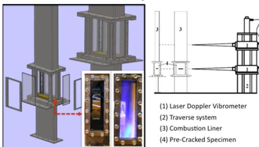
Figure 2 : Vibration-based monitoring on combustor.
