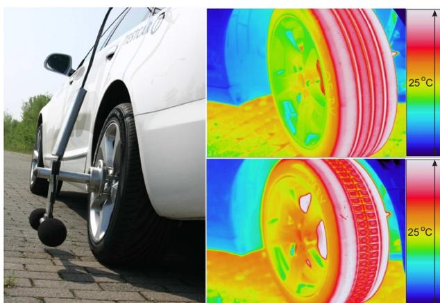
Figure 1 : Experimental setup mounted on the car (left) and infrared pictures of the grooved tyre (above) and block pattern tyre (below) to indicate the temperatures.
