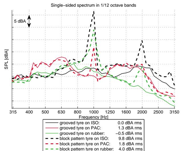
Figure 2 : Normalized experimental sound pressure levels of the front microphone at 100 km/h.
