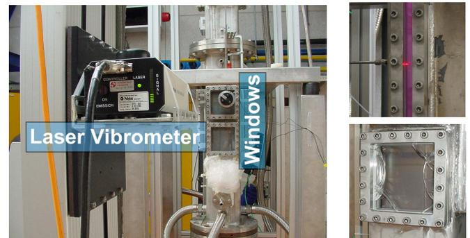
Figure 3 : Laser vibrometer measurements on the liner.
