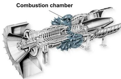
Figure 1 : Siemens V94.3a gas turbine
