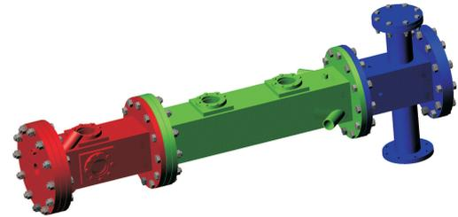
Figure 2 : Concept for test rig, red = PLIF measurements, green = structural measurements, blue = water-cooler
