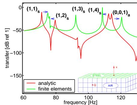
Figure 3 : Transfer volume source to displacement
