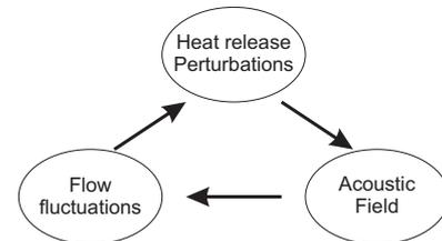
Figure 2 : Thermoacoustic feedback
