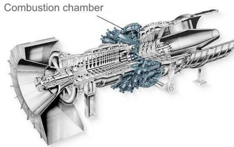
Figure 1 : Combustion chamber in Siemens gas turbine
