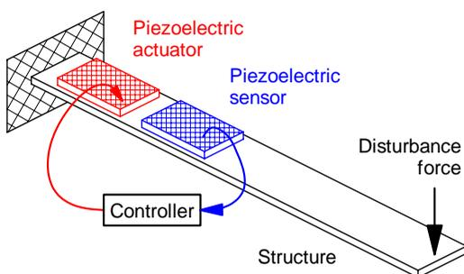
Figure 1 : Beam with piezoelectric sensor and actuator
