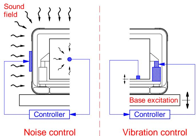
Figure 3 : Active control of noise and vibration
