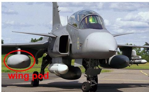
Figure 1 : Fighter aircraft with wing pod
