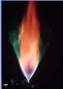
Figure 1: A methanol spray flame
