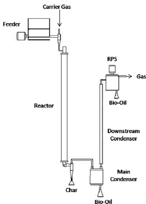
Figure: Schematic of the experimental setup
