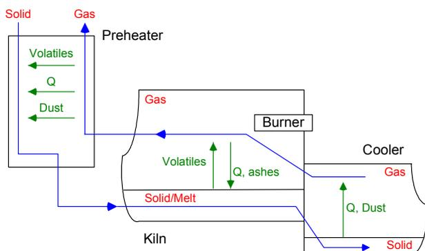
**Figure 1.** Mechanism of the kiln-cooler interaction.
