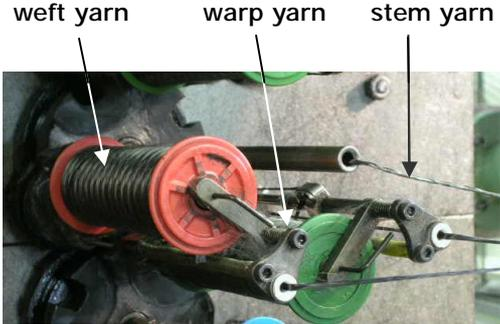
Figure 2. Yarn supply in the spool plane.
