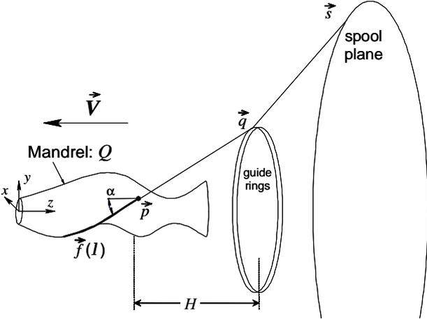
Figure 3. Model of a braiding machine with a complex mandrel.
