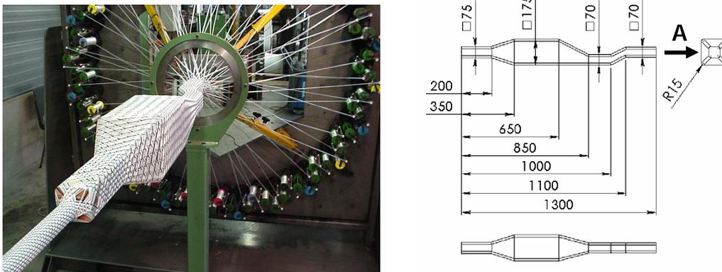
Figure 7. Validator mandrel; left: in the braiding machine, right: mandrel dimensions.
