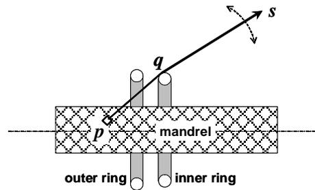
Figure 6. Position of the supply point  $q$  between the spool position  $s$  and the fell point  $p$ .
