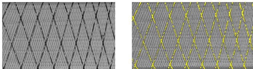
Figure 8. Image analysis using the highlighted yarns for fibre orientation measurement.
