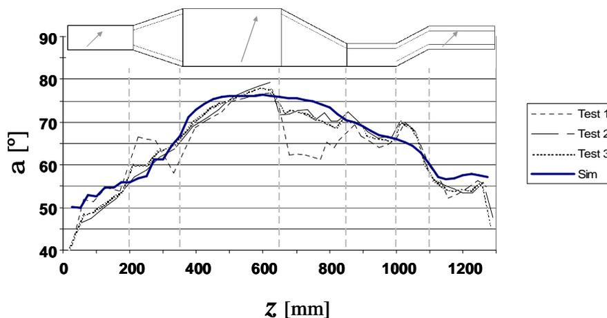
Figure 9. Braid angles (warp) vs  $z$ -coordinate on face A (fig.7): experimental and simulation results.
