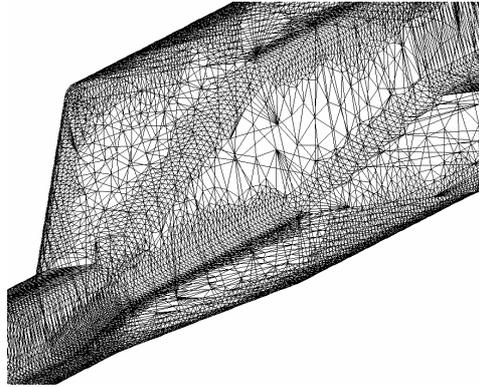
Figure 4. Triangular surface mesh of a mandrel surface.
