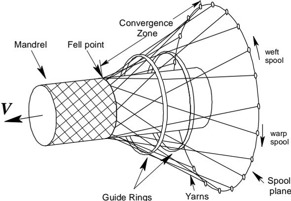
Figure 1. Braiding machine (schematically).
