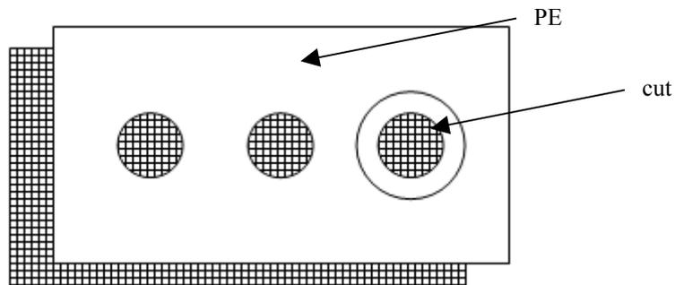
Fig 5 PE film on the fibre mat
