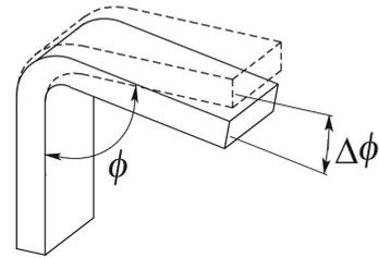
Fig. 1. Decrease of the enclosed angle of an L-shaped part
