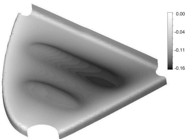
Fig. 4. Vertical displacements (mm) caused by spring-forward
