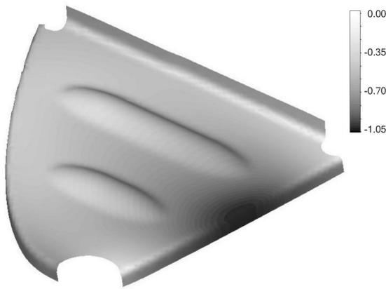
Fig. 3. Vertical displacements (mm) caused by thermal membrane stresses
