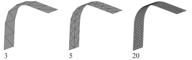
Fig. 2. L-shaped strip meshed with 3, 5 and 20 elements over the arc radius, respectively
