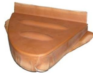
Fig 3: Wing leading edge stiffener
