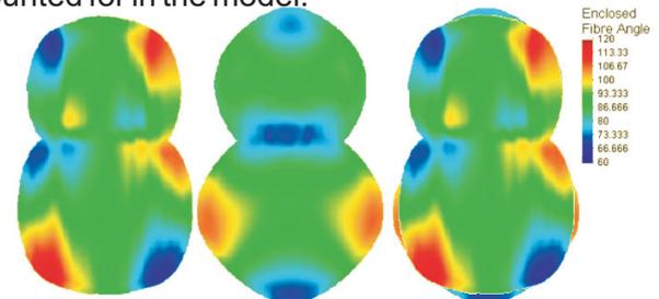
Figure 3: Drape modeling of the product,  $[0/90]_{2s}$  cross-ply,  $[45/-45]_{2s}$  cross-ply and QI  $[0/90 | 45/-45]_s$  laminates
