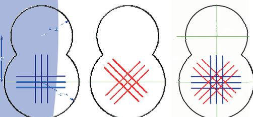
Figure 2: Fibre orientations for  $[0/90]_{2s}$  cross-ply,  $[45/-45]_{2s}$  cross-ply and QI  $[0/90 | 45/-45]_s$  laminates
