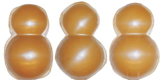
Figure 4: Experimental drape results for  $[0/90]_{2s}$  cross-ply,  $[45/-45]_{2s}$  cross-ply and QI  $[0/90 | 45/-45]_s$  laminates
