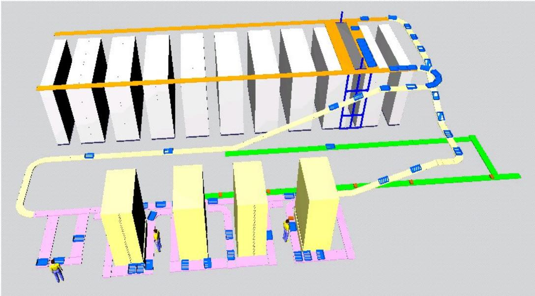
Figure 4: The integral Logistacker orderpicking system and its environment: the Logistacker (at the top), the internal transportation system and the orderpick work stations (at the bottom).
