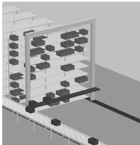
Figure 2: First version of the Logistacker with the liftable conveyor positioned at the I/O level, where the fixed external conveyor is situated.
