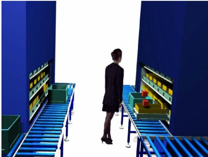
Figure 5: Orderpick work station consisting of tandem carousels, operated by one orderpicker
