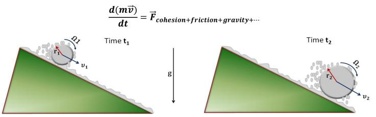
A cohesive ball rolling down an inclined plane at time  $t_1$  (left fig.) and at time  $t_2$  (right fig.) with increased radius
