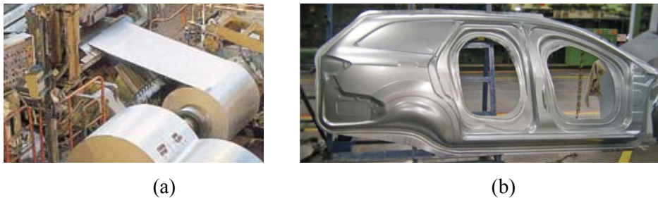
Figure 1.1: (a) Skin pass cold-rolling mill with EDT surface texturing (Source - Tata Steel website) and (b) Side panel of Ford Mondeo car (Source - Corus Emotion, issue 14, 2008).
