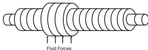
Figure 1 : Flow forces applied to structure model
