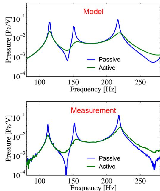
Figure 4: Predicted and measured acoustic response.
