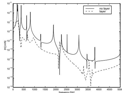
Figure 4 : FRF of top of the housing in vertical direction
