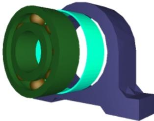
Figure 1 : Viscoelastic layer mounted between the bearing and the housing
