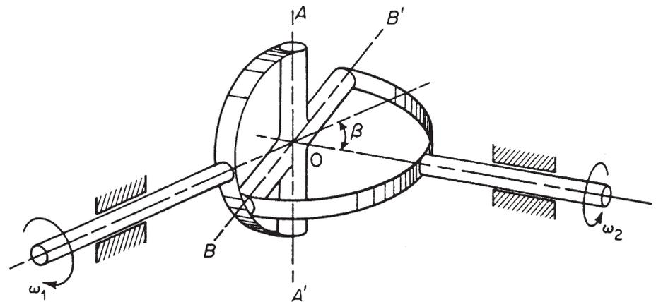
Cardan-joint (machine component)
