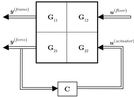
The outputs are defined in two parts as well. The first part contains the output-signals of so-called performance acceleration sensors which are attached at nodal points 3, 5, and 7. These accelerations are included in the output vector
