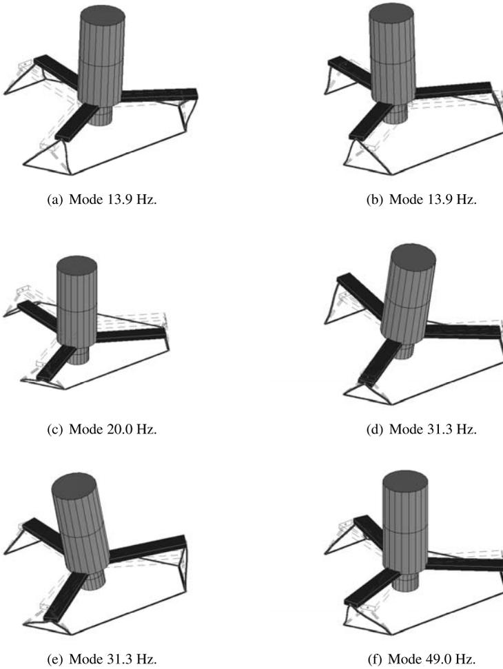
**Fig. 9** Mode shapes and natural frequencies of the passive system
