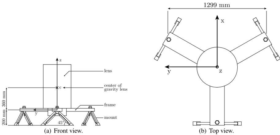
**Fig. 4** Front and top view of the metrology frame
