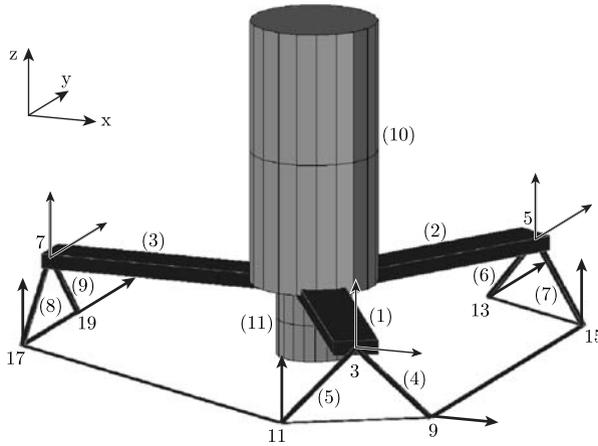
**Fig. 7** Finite element model of metrology frame and floor using beams
