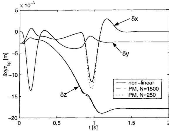
Figure 13. Deviation from the nominal tip trajectory according to a non-linear simulation and from the perturbation method (PM) using 250 and 1500 linearization points  $N$ , respectively.
