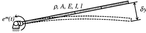
Figure 4. Elastic beam attached to a hub rotating about an axis fixed in space.
