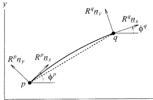
Figure 1. Planar flexible beam element.
