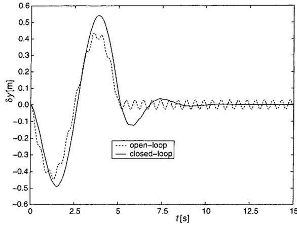
Figure 7. Tip-deflection  $\delta y$  using the perturbation method for a trajectory motion without controller (open-loop) and for controlled trajectory motion (closed-loop with  $\omega = 1.45$  rad/s and  $\beta = 0.9$  in Equation (37)).
