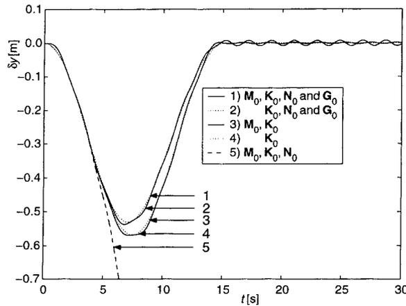
Figure 5. Tip-deflection  $\delta y$  for spin-up motion using different perturbation approximations.
