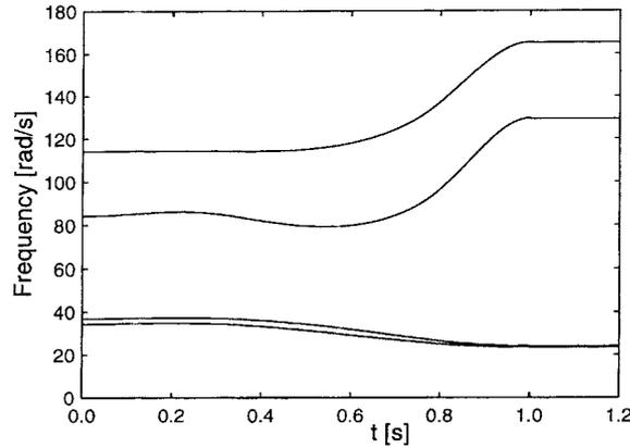
Figure 11. Four lowest constrained natural frequencies during the manipulator motion.
