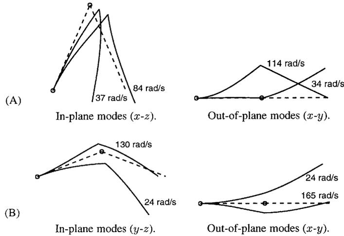
Figure 12. Constrained mode shapes in initial (A) and final (B) configurations.
