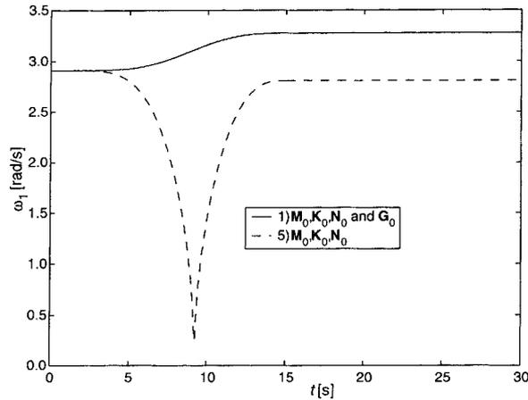
Figure 6. Time dependent natural frequency  $\omega_1$  of the first constrained bending mode.
