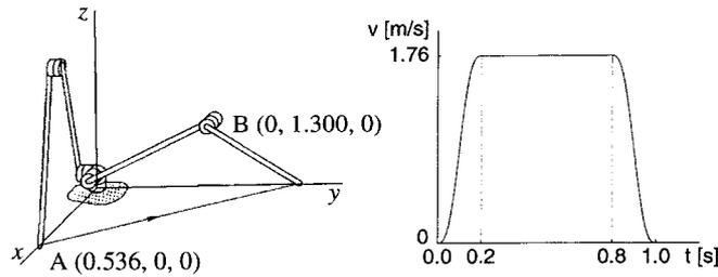
Figure 9. Motion trajectory and velocity profile of manipulator tip.
