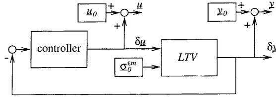
Figure 3. Block diagram of a typical closed-loop simulation in SIMULINK based on the perturbation method.
