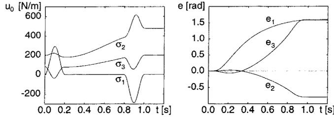
Figure 10. Nominal actuator moments applied at hinges (1), (2) and (3) and the nominal relative rotations of the hinges. The rotations  $e_1$ ,  $e_2$  and  $e_3$  are relative to their initial positions.
