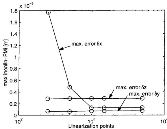
Figure 14. Maximum errors in the coordinates of the tip position as functions of the number of linearization points. The error is defined as the difference in each coordinate between the perturbation method (PM) and the non-linear simulation.
