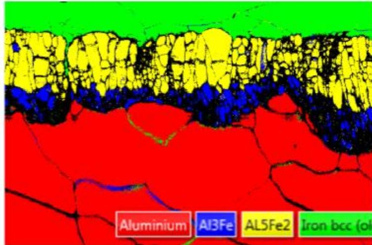
*Al layer deposited on top of steel*
